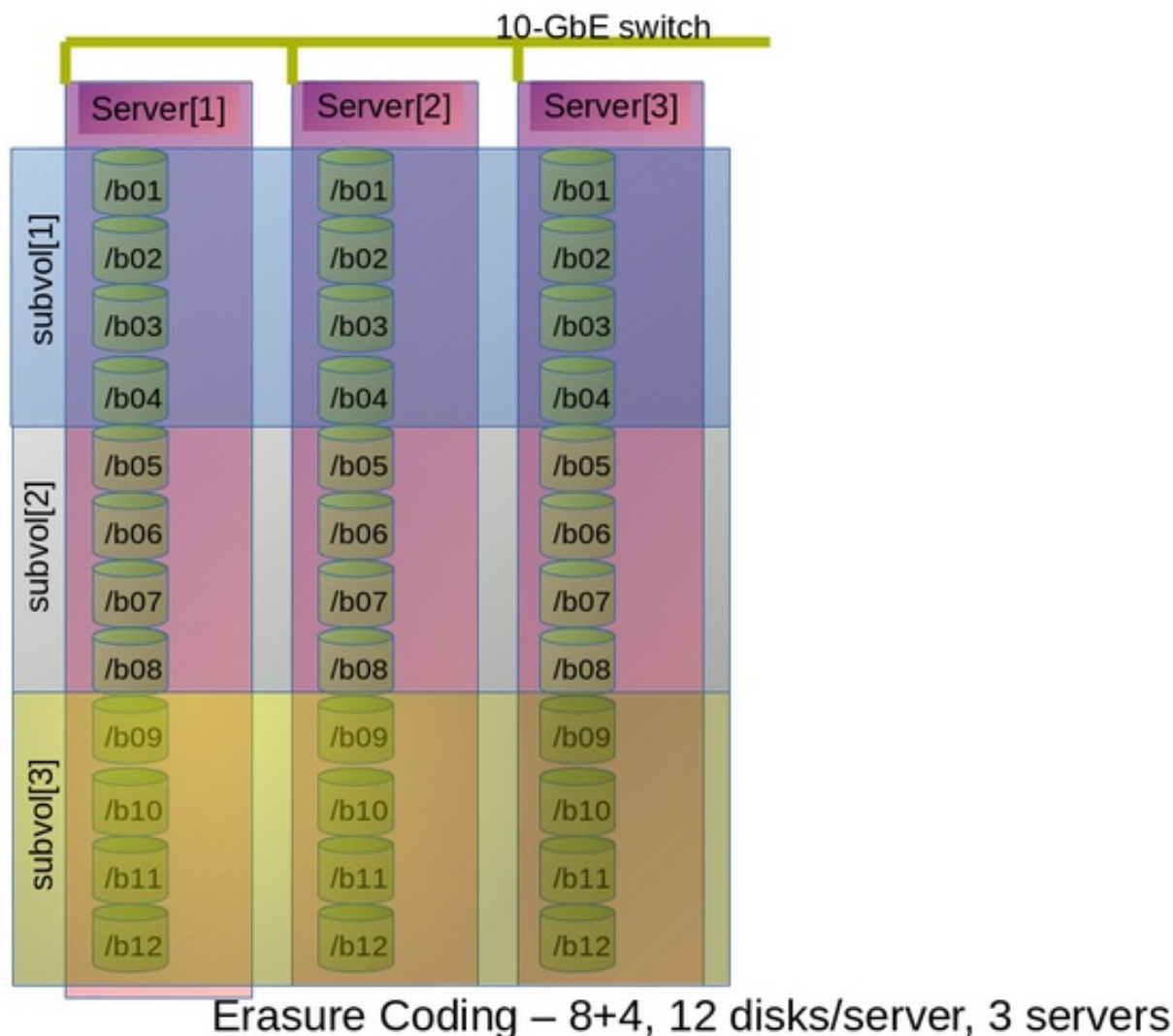
Figure 11.1. Example Configuration of 8+4 Dispersed Volume Configuration
