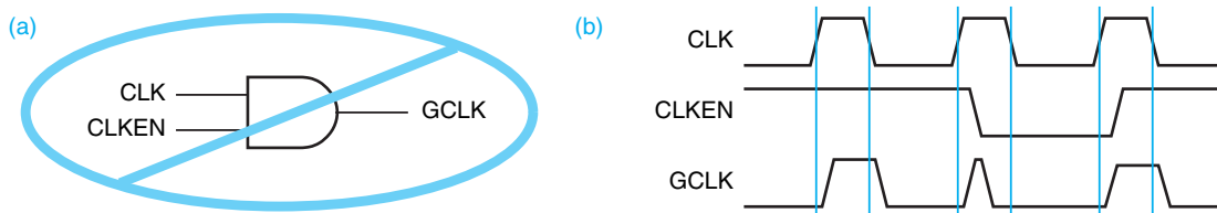
Figure 13-12 Bad clock gating: (a) simple-minded circuit; (b) timing diagram.
