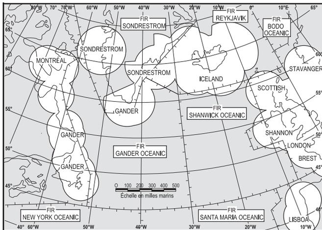
**Figure 2.3 – Couverture VHF NAT à 30 000 pi**
