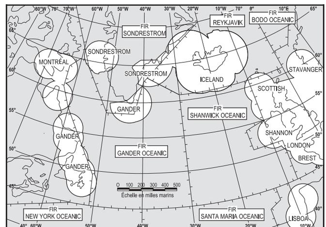
**Figure 2.2 – Couverture VHF NAT à 20 000 pi**
