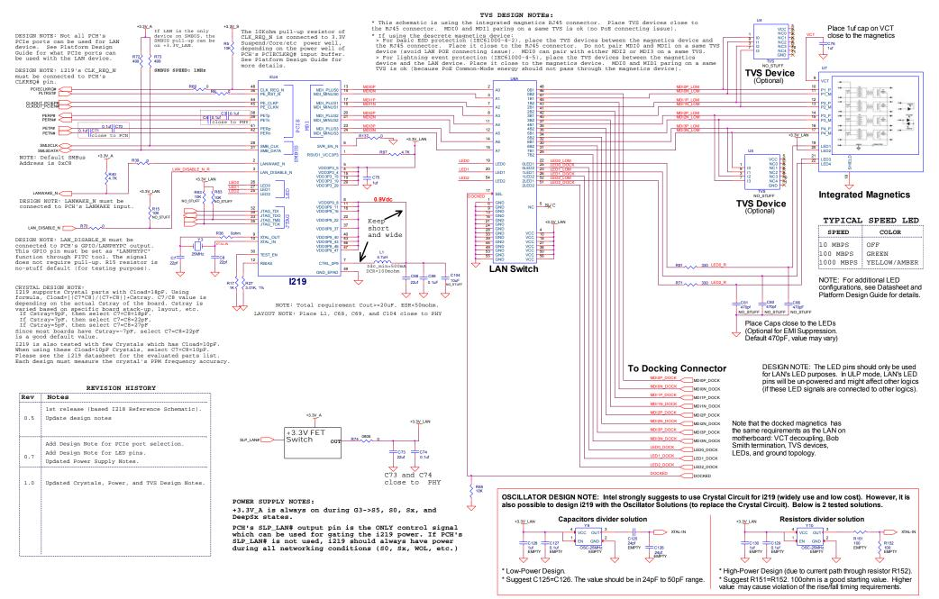
NOTE: This is a typical Mobile Docking Design. For designs without a docking connector, the lanswitch device is not necessary so it can be removed. Please see the schematic/layout checklist for details.
