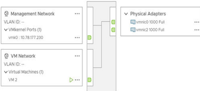
Figure 2-2. Topology Diagram of a Standard Switch That Connects the VMkernel and Virtual Machines to the Network
