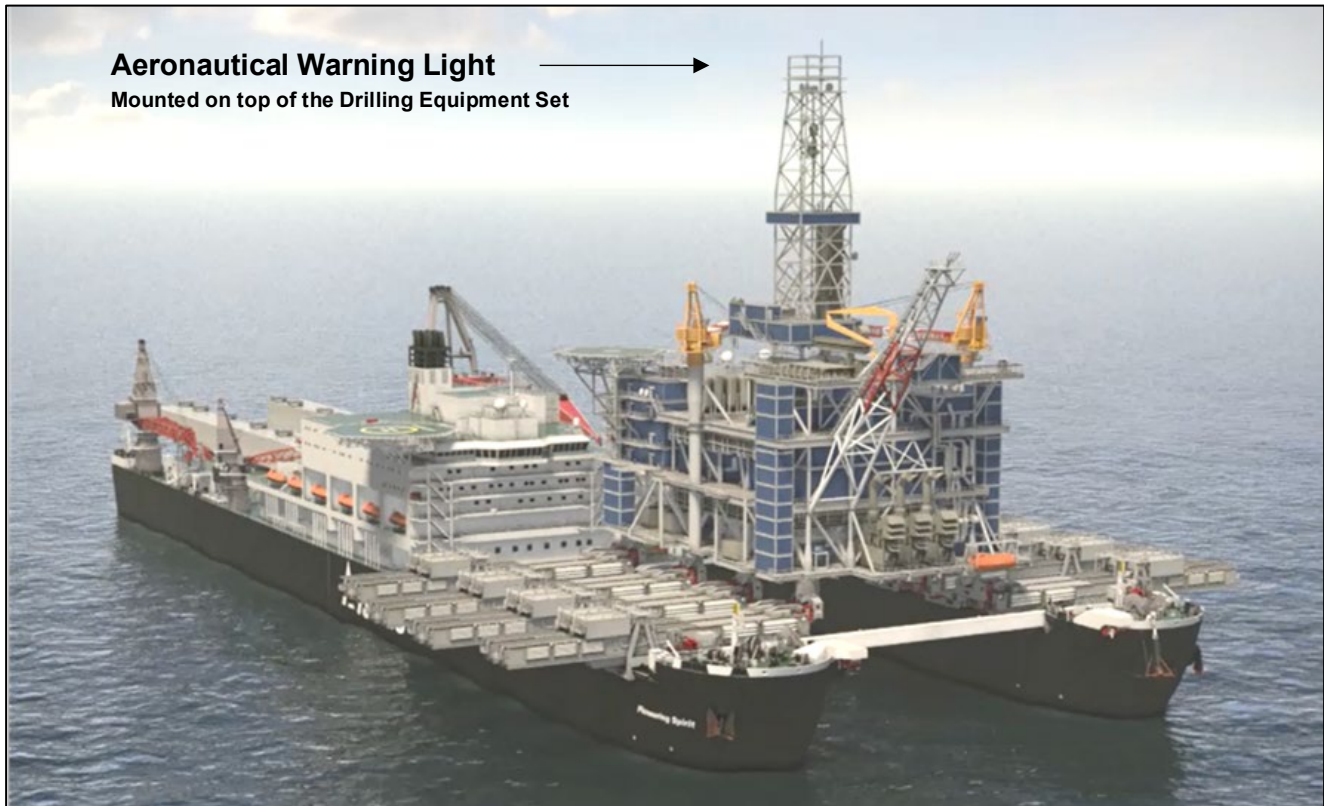
Figure 2. Topsides Structure on the Installation Vessel “Pioneering Spirit”
