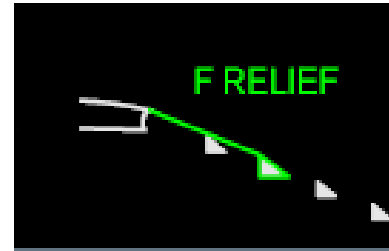
The Flap Load Relief Function is active. The indication pulses.
